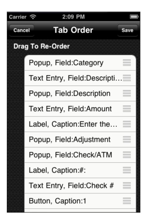
To adjust the tab order, select Adjust Tab Order from the Tools button. Here you will see a list of all the controls on the form. You can drag the right icon up or down to re-order as necessary.
